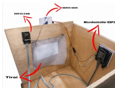
Gambar 2. Implementasi prototipe sistem kendali tirai otomatis berbasis gesture recognition
